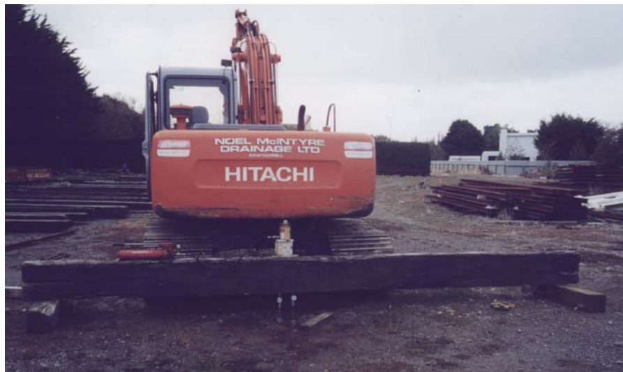
Figure 1. Beam test setup
